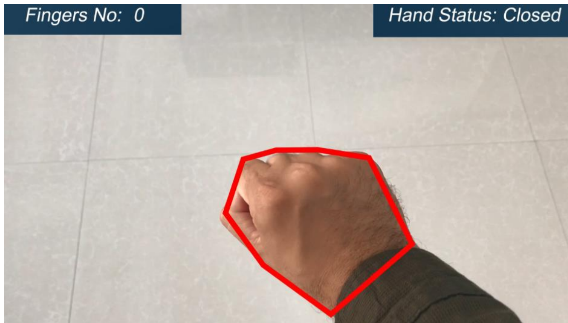
Figure 4.8 : Closed Hand Pose Detected by our system, and at the top we can see fingers numbers and hand status
