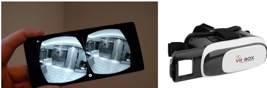
Figure 3.6 : Right Figure shows google cardboard VR glasses, and the left one shows the divided VR screen
