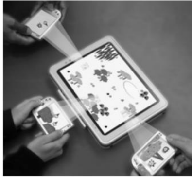
Figure 2.8 : In this illustration, three students are depicted inspecting regions of the MUSHI simulation. The simulation, running on a tablet PC, wirelessly delivers content to their handhelds
