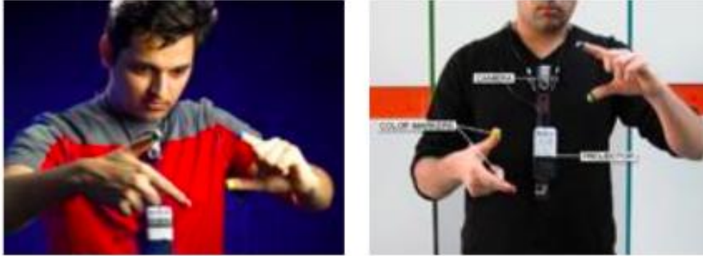
Figure 2.4 : six sense device which is wearable on human chase which showing the projector and camera
